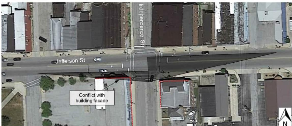
Figure 7 – Sight Distance Triangles for Northbound Independence St.
